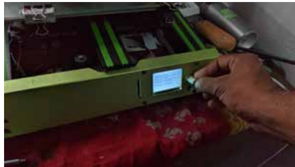
Step 2: Put printer into pre-heat mode - this is done to melt the filament in the hotend to help remove nozzle without damaging components
