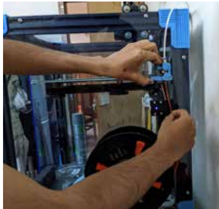
Step 7: Push the filament all the way through till hotend
