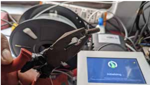
Step 5: Removed nozzle is then cleaned using alcohol and brush and put back in a similar manner
