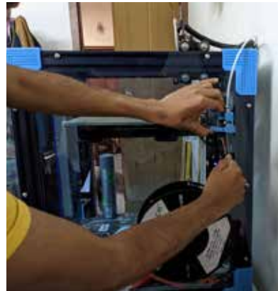
Step 3: Press onto the extruders spring tensioner and pull filament out. The tensioner is left handed.
