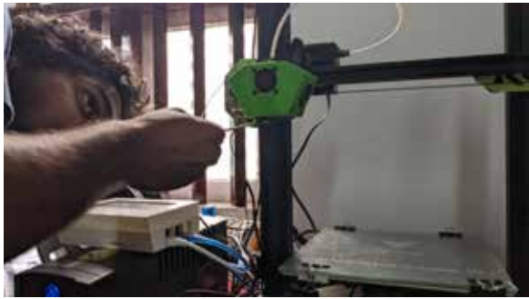
Step 3: Using a spanner to remove the hot nozzle
