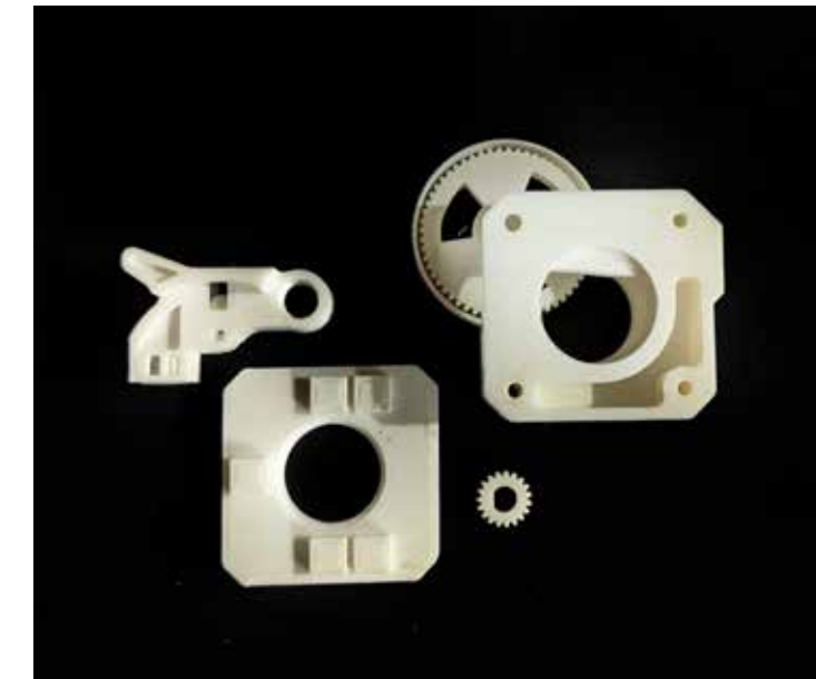
Prototype of a gantry plate printed on PLA was made to test the functionality of such a module. The prototype is strong and can hold the weight of the extruder without an issue
