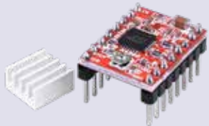
A4988 is an inexpensive stepper driver module that does the work but produces a lot of noise
