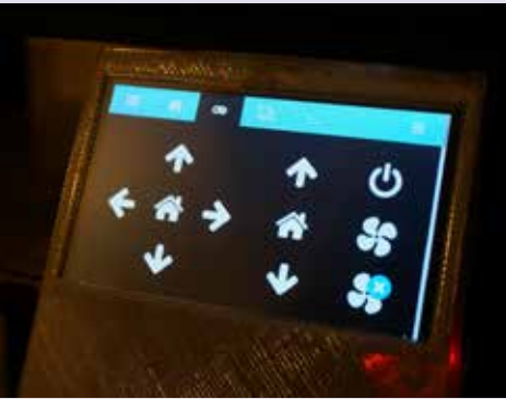
Touch screen interface on Klippper. Klipper lacks support for older interfaces
