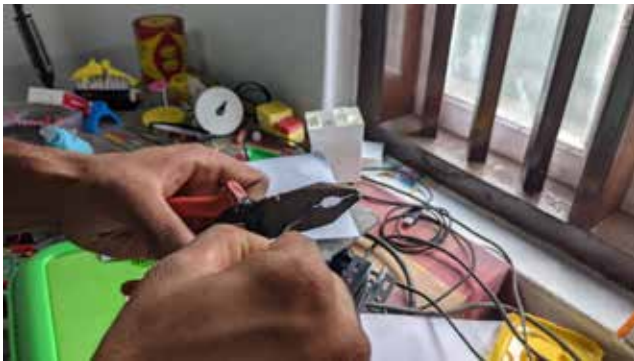
Step 4: Cuts end of filament for easier changing
