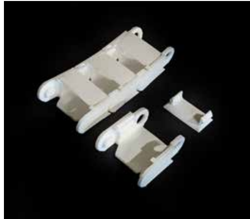
Prototypes of a drag chain for wire management. Makes use of two printed parts that can be connected together to the desired length. This approach is time consuming and cost-inefficient. The economical alternative is PVC wire harness tubing.
