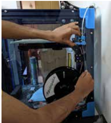
Step 4: Tries to put in new filament, doesn't go in because of blunt rounded ends from melting
