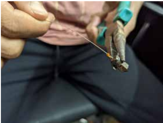
Step 4: Leftover filament in the nozzle is pulled out along with the needle
