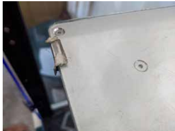
Glass bed clips loose over time fixed with tape
