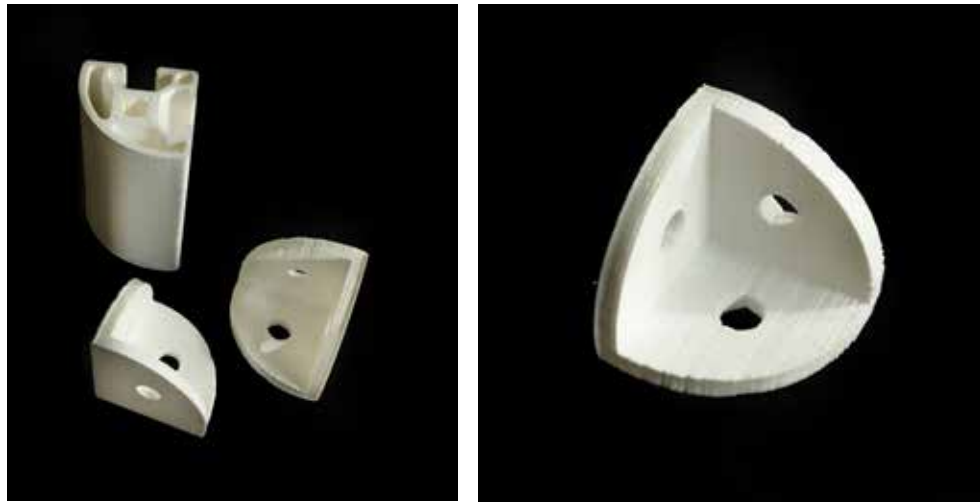
Final prototypes of Corner Connectors - since 2020R profiles weren't available a 3D printed version was used to check compatibility and was found satisfactory
