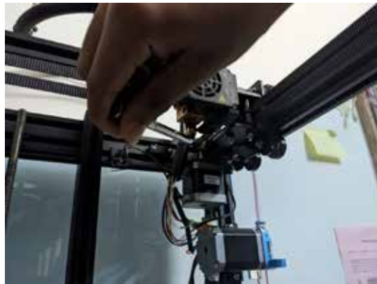
Step 1: Remove the nozzle with a wrench. This takes a lot of fiddling due to inaccessibility in this particular printer
