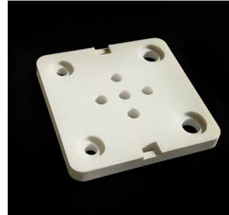
Prototype of a gantry plate printed on PLA was made to test the functionality of such a module. The prototype is strong and can hold the weight of the extruder without an issue
