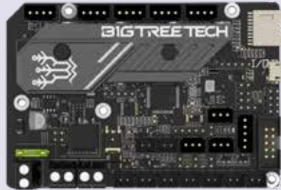
BIGTREETECH SKR E3 Mini V3 is a level up board for most budget 3D printers - it is not the cheapest but is incredible value for money because of the silent drivers and 32-bit processor
