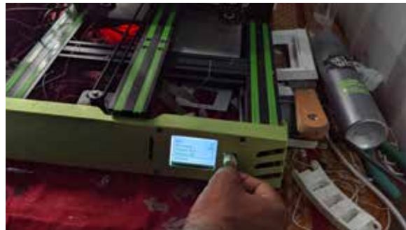
Step 4: Printer is put into cooldown mode - to cooldown the half-unbolted nozzle
