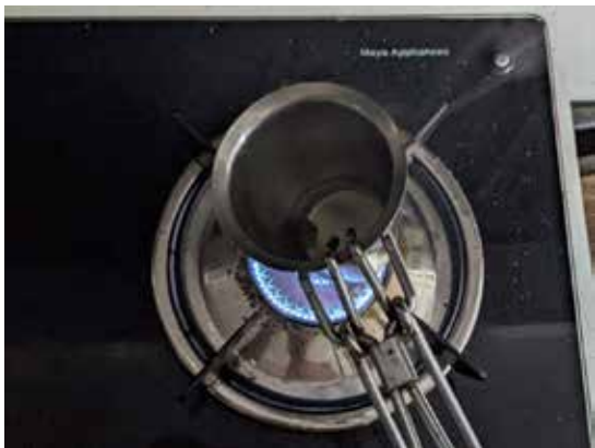
Step 6: Immersed in cooking oil, the nozzle is heated, this forms a layer of solidified oil around the nozzle preventing filament from sticking onto nozzle - this is a common procedure and is done with many different types of oils
