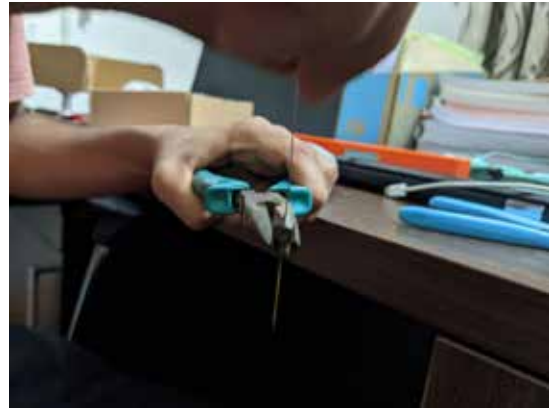
Step 3: nozzle cleaner needle is inserted into the nozzle
