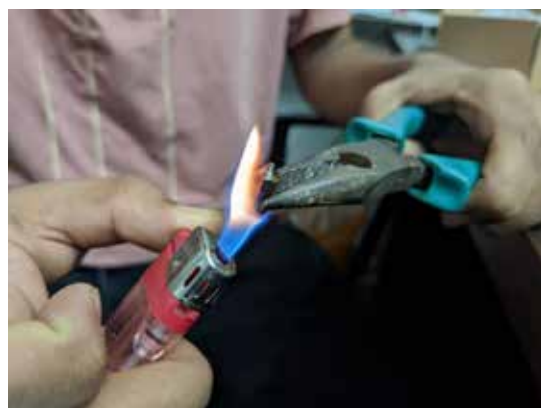
Step 2: Heat the nozzle to melt leftover filament and residue
