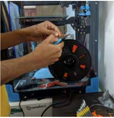
Step 5: Cuts the end of filament for cleaner sharper edges
